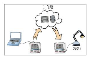
The Internet of Things describes devices that are connected to the Internet. Data is sent and received via built-in sensors. In this course, data is sent from the Micro:bit transmitter to a network server. The server then forwards the data to the Micro:bit receiver, which causes the IoT device to turn on and off.
